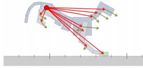
Figure 5: The character features consist of the displacements of the centers of mass of all links relative to the root (red) and their linear velocities (green).
