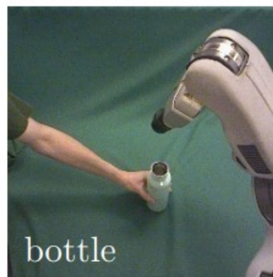
Figure 1: Our method learns visuomotor policies that directly use camera image observations (left) to set motor torques on a PR2 robot (right).
