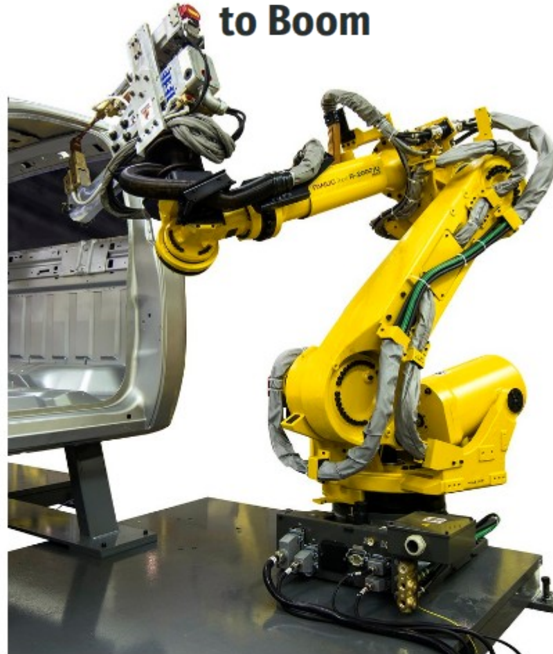
A Fanuc R-2000iC robot spot-welding the body of a truck. Photo: Courtesy of Fanuc
