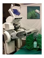
amount of training data, distractors that are correlated with task-relevant variables can hamper generalization. For this reason, the left arm is covered with cloth to prevent the policy from associating its appearance with the object's position.
