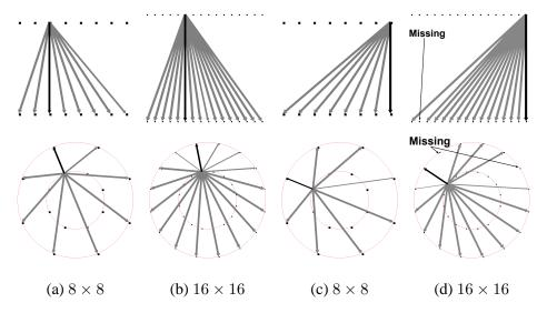
Figure 16: **Perfect and Imperfect Scaling.** The parallel (top row) and concentric (bottom row)  $8 \times 8$  motifs in (a) scale perfectly to the  $16 \times 16$  motifs in (b). However, because of artifacts at higher resolution, not all motifs scale perfectly, as shown between (c) and (d), in which missing connections are identified by arrows. While the motif is mostly intact, slight imperfections of this type are common during scaling in this task.
