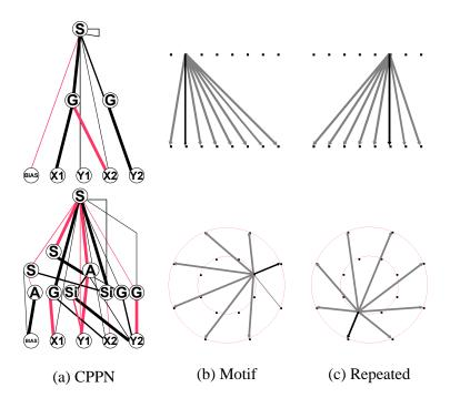
Figure 15: **Repeated patterns in solutions.** The CPPNs in (a) represent parallel (top row) and concentric (bottom row) substrates that solve the task. The connectivity patterns in (b) and (c) are outgoing *motifs*, each from a single input node in the substrate. These images show that the same motif is repeated in different locations.
