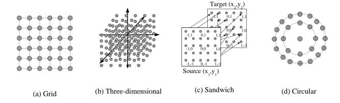
Figure 6: Alternative Substrate Configurations. This figure shows (b) a three-dimensional configuration of nodes centered at (0,0,0), (c) a "state-space sandwich" configuration in which a source sheet of neurons connects directly to a target sheet, and (d) a circular configuration. Different configurations are likely suited to problems with different geometric properties.
