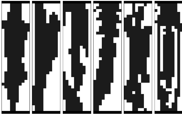
Figure 6: Six examples of stereotypical structures evolved for Random Frequency Profile #1. Black pixels represent stiff material, while white pixels represent soft material. Optimized structures often consist of one or two large continuous regions. They often span all or nearly all of the design space allocated in both width and length. They also often display minor branching structures off of this primary long-spanning structure.
